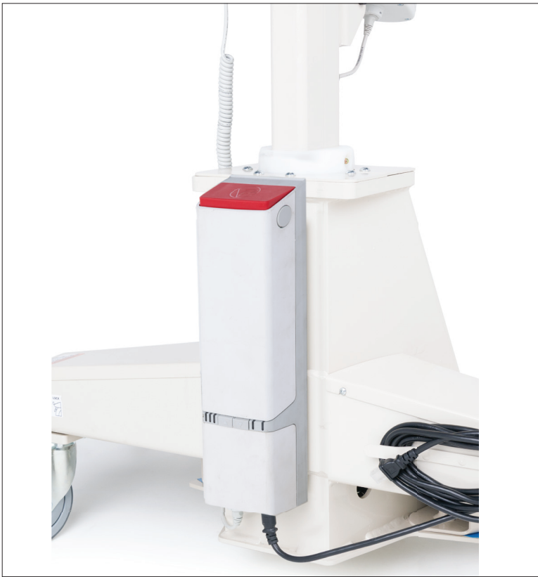
Red Emergency Power-Off Button
